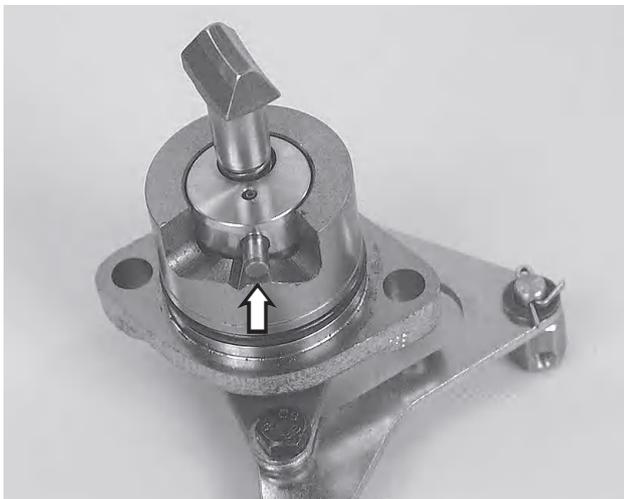
11. Put the gear shift mechanism in a position between forwards and neutral. The pin should rest in one of the “notches”.
