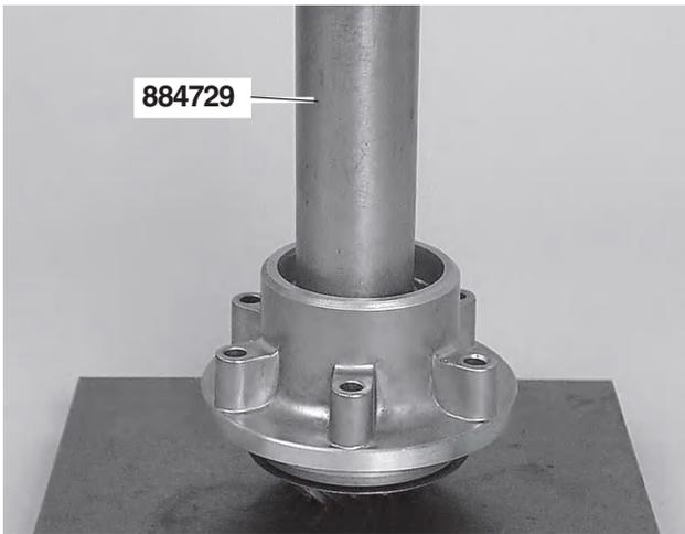
**39.** Place the drive shaft in the bearing housing and press the small roller bearing on, using tool no. **884729**.
