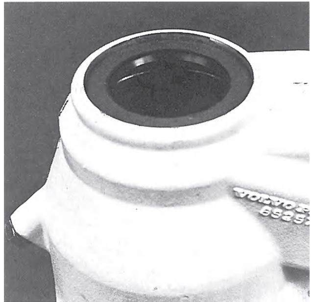
**22.** Apply sealant, Volvo Penta part no. 1161099-5 to the gearbox housing and install a new seal ring. Use tool no. **884834** and shaft **884859**.
