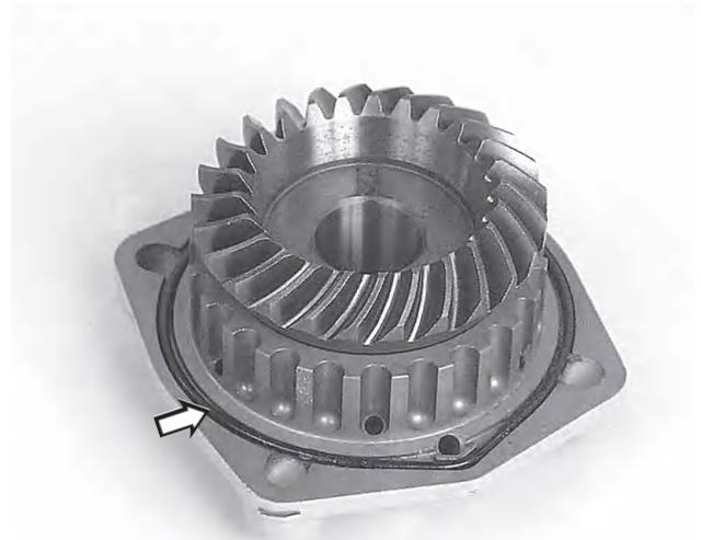
**111.** Put a new O-ring in the groove in the upper bearing housing. Then install the bearing housing on the housing.
