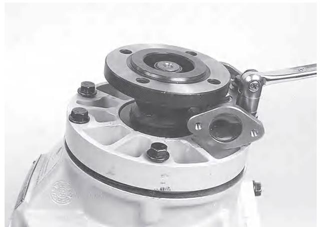
**84.** Put in shims of the calculated thickness, plus a further 0.5 mm in the cover and install the bearing race. Put a plate on the bearing race and press.
