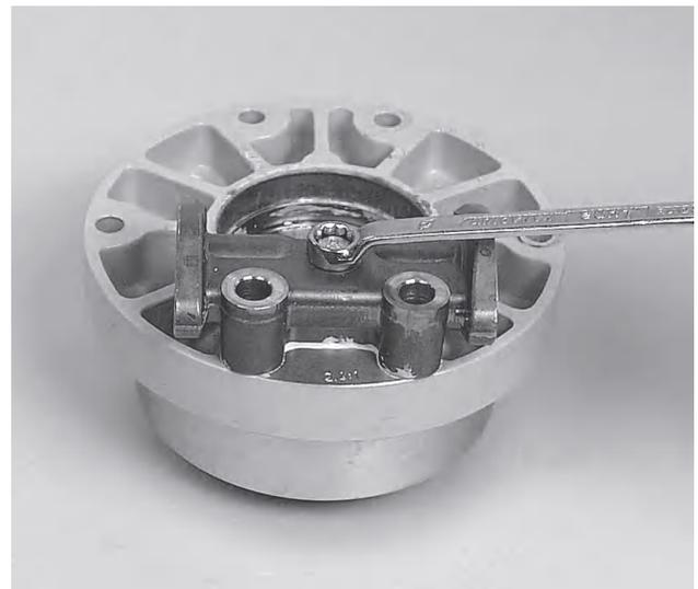
65. Apply sealant, Volvo Penta part. no. 840879-1 on the mating face against the bearing housing.
