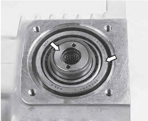
81. Put the slipping clutch into the housing and place the outer bearing race loose on top of the bearing.
