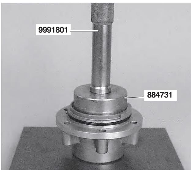
36. Press the large outer bearing race into the bearing housing. Use tool no. **884731** and shaft **9991801**.
