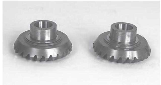
**48.** Put shims on the gear wheels for the upper bearing housing and gear housing. Start off with 0.50 mm for each gear wheel. This is a value which is based on experience.
