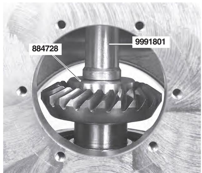
**49.** Press the gear wheel into the gear housing. Use tool no. **884728**, shaft **9991801** and **884739** as a support for the inner race.
