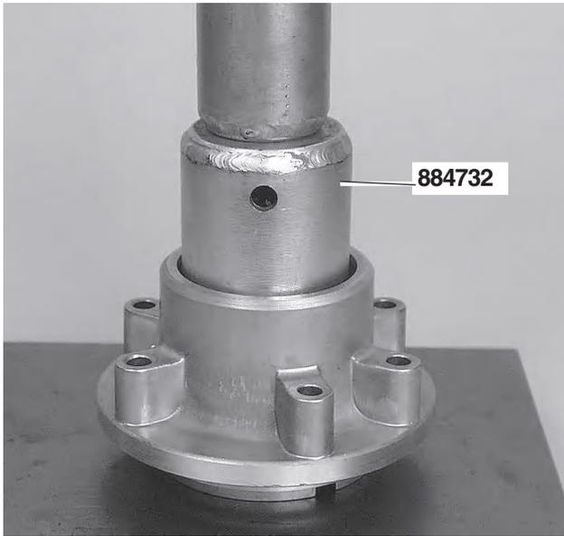
35. Press the small outer bearing race into the bearing housing. Use tool no. **884732**.
