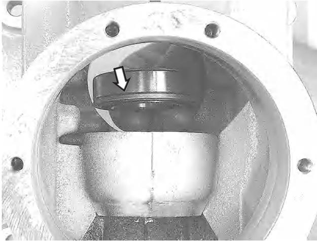
96. Install the lower roller bearing in the housing.
