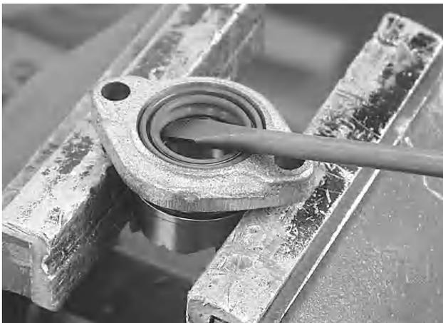
7. Remove the seal ring with a screwdriver. Clean all components of the gear shift mechanism and check for wear. Change components as necessary.
