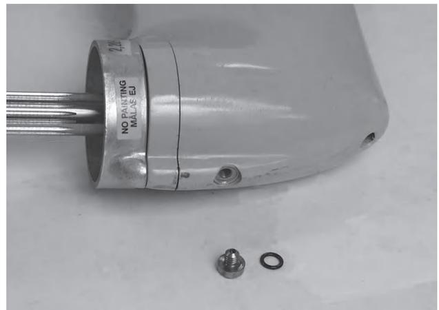
77. Change the gasket on the oil drain plug.
