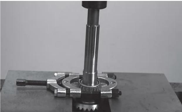
**21.** Remove the **rear** roller bearing. Use a knife extractor as a counterhold, with a **17 mm** socket on the shaft end.
