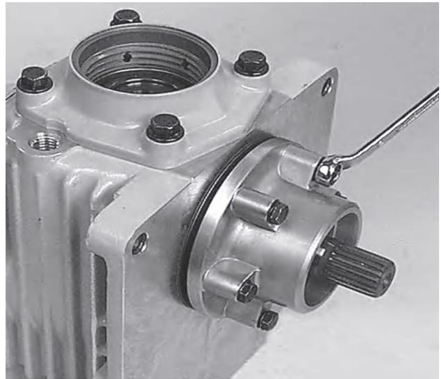
98. Try installing an 0.40 mm shim in the input bearing housing.
