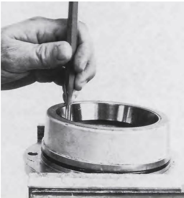
10. Remove the seal ring from the cover. The seal ring must always be replaced by a new one.
