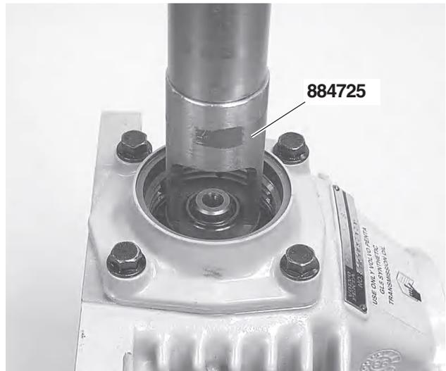
**114.** Press down the large washer so far that the retaining ring halves can be put in the groove.
