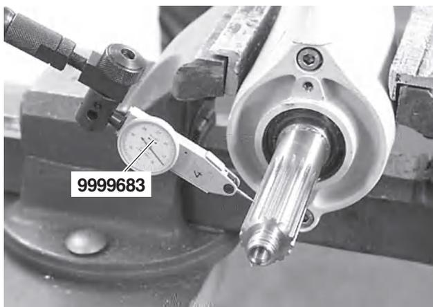
**51.** When the highest torque specified above has been reached, the gear housing should be removed from the vice and fixed vertically instead. Let the tool remain on the gear housing.
