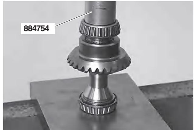
**32.** Press the rear roller bearing down onto the propeller shaft. Use mandrel **884754**.
