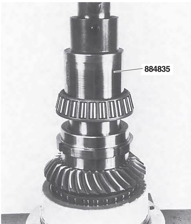
**29.** Press the outer roller bearing on. Use sleeve **884835**.
