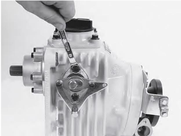
1. Disassemble the gear shift mechanism, 2 screws.
