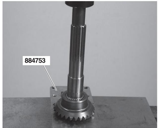
**22.** Remove the gear wheel with tool no. **884753**. Use a socket to protect the end of the shaft.
