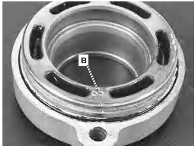
**35.** There is a dimension (**B**) punched on the rear bearing housing. This dimension is stamped underneath the bearing housing, and varies between 50-70. In this case, the distance is 65 mm.
