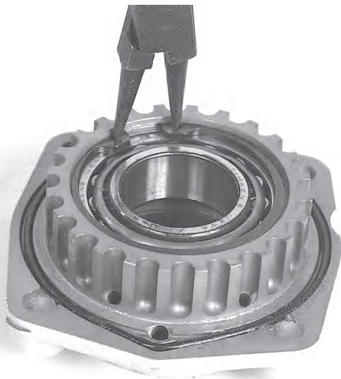
44. Remove the circlip, using circlip pliers.
