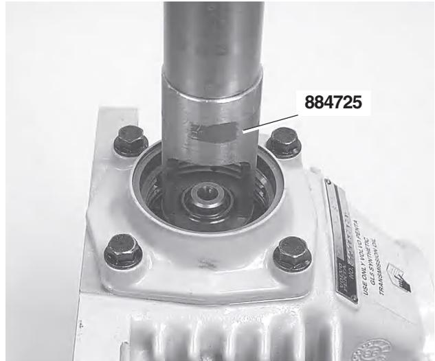
**20.** Turn the reverse gear/upper bearing housing over and put it in a press. Put tool no. **884725** over the vertical shaft, so that it rests on the large washer. Press the washer down, to release the retention ring halves. Remove the halves.
