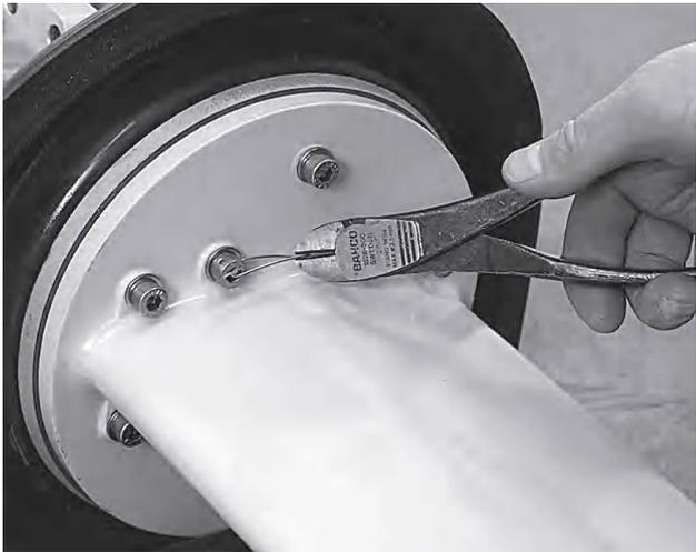
2. Remove the locking wire from the four screws. Then remove all the screws, 10 pcs below the division line of the drive.
