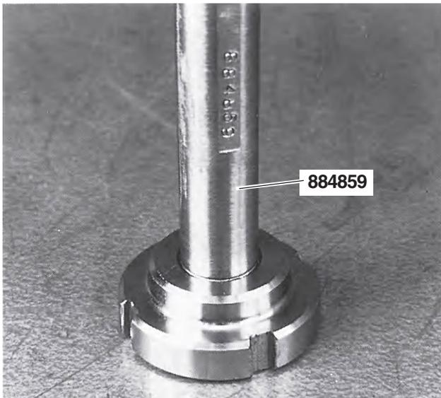
**21.** Install a new needle roller bearing in the pinion nut, using mandrel **884859**.
