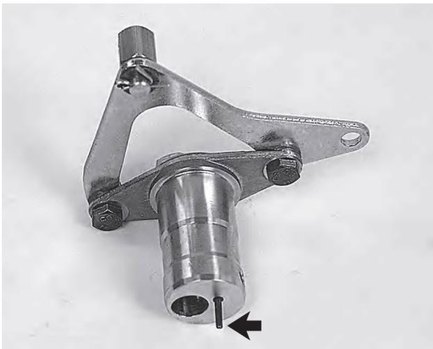
6. Shake the pin out of the eccentric piston.
