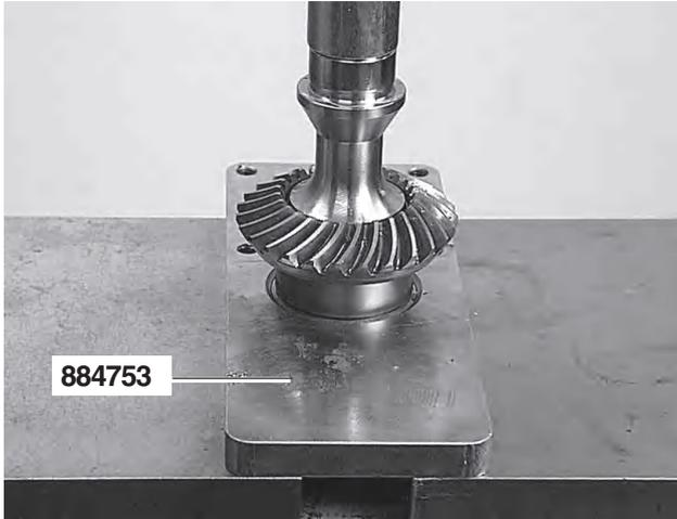
24. Press the gear wheel down to the step on the propeller shaft with tool no. **884753**. Make sure that it seats securely.
