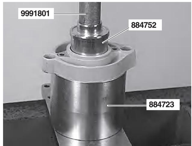
**23.** When the seal rings are changed, the outer bearing race should also be changed.
