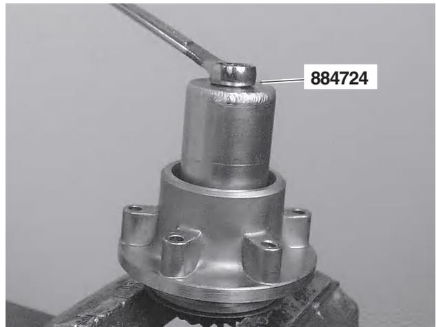
30. Fix the gear in a vise. Use soft facings on the vise jaws. Then disassemble hook nut with tool no. **884724**.
