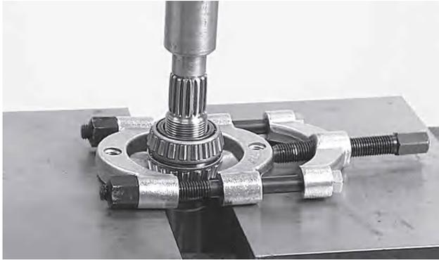
14. Remove the roller bearings with a knife extractor as counterhold. Use a hydraulic press together with a suitable mandrel.
