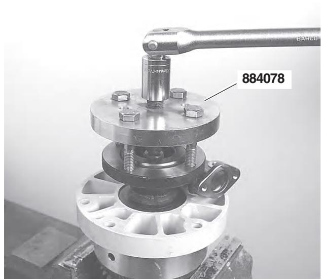
53. Disassemble the propeller shaft flange. Use tool no, **884078**, wrench dimension **19 mm**, or a claw puller.
