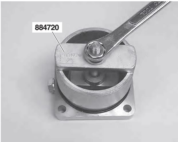
**92.** When the correct flank clearance and marking pattern have been obtained, disassemble the output bearing housing, lower bearing cover and slipping clutch.
