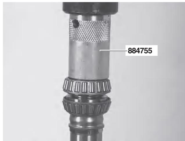
19. Install the other roller bearing inverted, i.e. with the smaller end upwards. Use mandrel **884755**.
