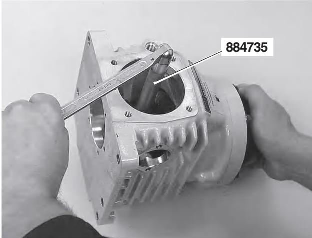
**88.** Remove the output bearing housing and apply a thin layer of marking dye to the lower gear and the gear wheel on the output shaft.
