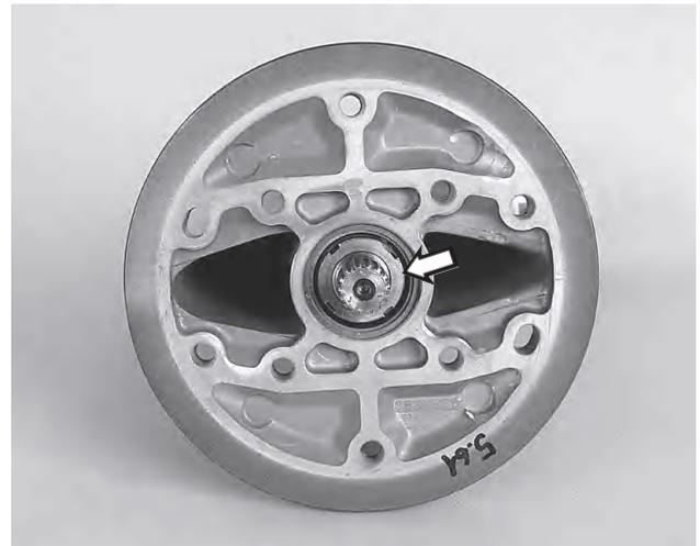
**48.** Install the upper nut on the vertical shaft.
