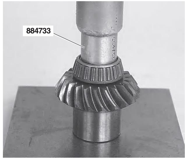
75. Press the small ball bearing onto the slipping clutch. Use tool no. **884733**.
