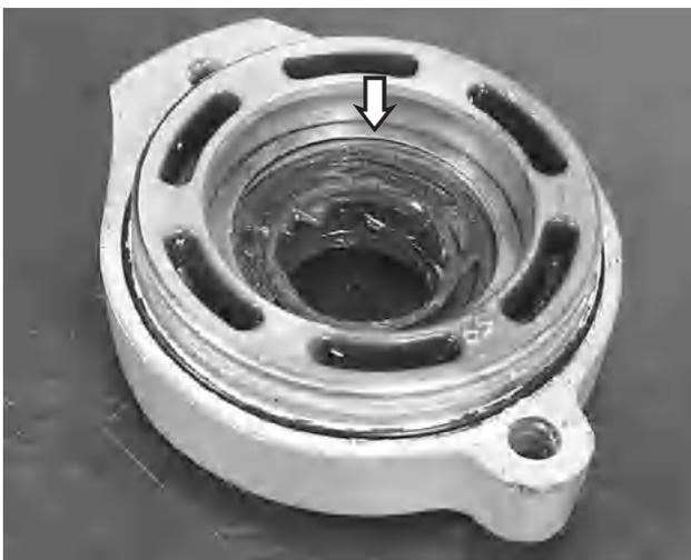
**39.** Put shims of the correct thickness in the bearing housing. In this case, they are 0.45 mm.
