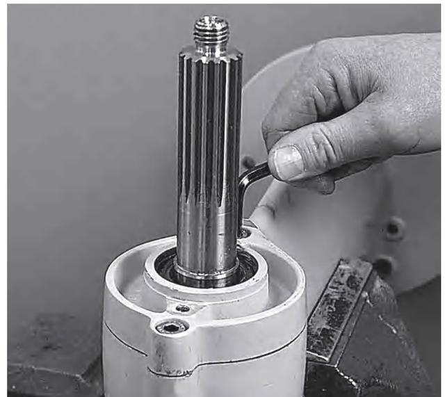
**41.** Install the propeller shaft in the gear housing.
