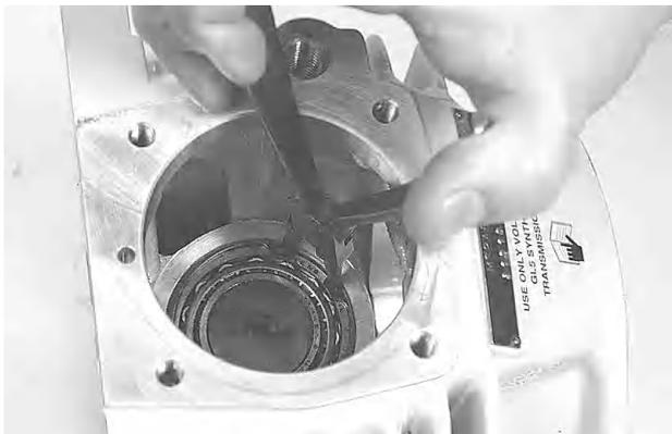
97. Install the circlip, using circlip pliers.
