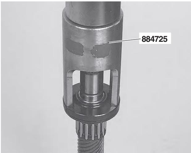
**108.** Put the shaft in a press.
