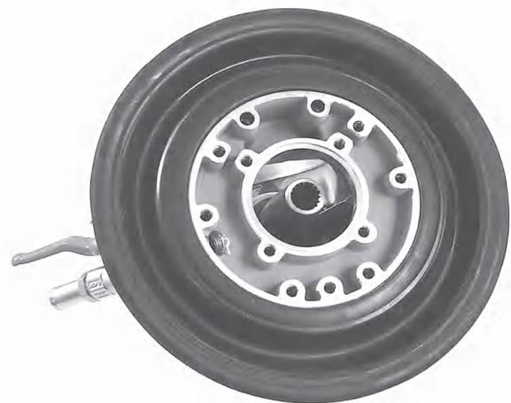
71. Put the rubber sleeve on the upper gear housing.
