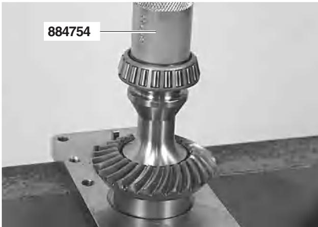
25. Install the front roller bearing with tool no. **884754**.
