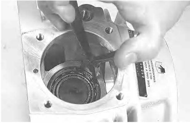
27. Remove the circlip, using circlip pliers.
