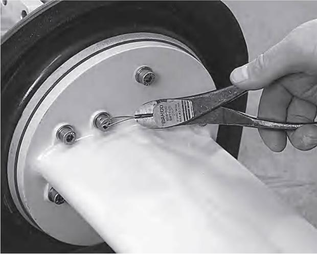
75. Secure four of the screws, the ones with holes in their heads, with locking wire, two screws on each side as in the illustration.
