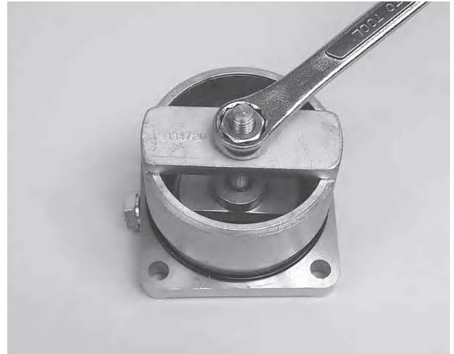
**70.** Put on O-ring (1) and thread seal ring (2) on.
