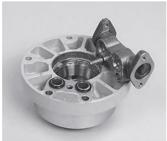
**61.** Remove the O-rings from around the cooling water pipe and screw hole. The O-ring for the screw hole is mounted on the screw.
