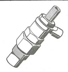
The fuel valve consists of injection nozzle and nozzle holder.
